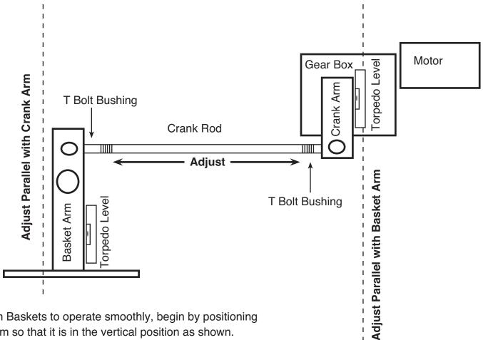
In order for the Curtain Baskets to operate smoothly, begin by positioning the Gearbox Crank Arm so that it is in the vertical position as shown. For proper adjustment position a torpedo level on the Crank Arm and Basket Arm as shown to ensure an EXACT horizontal level is achieved as shown. Adjust the Basket Arm position by twisting the T bolt bushing connected to the Crank Rod by either shortening or lengthening the Crank Rod until this vertical positions are achieved.
